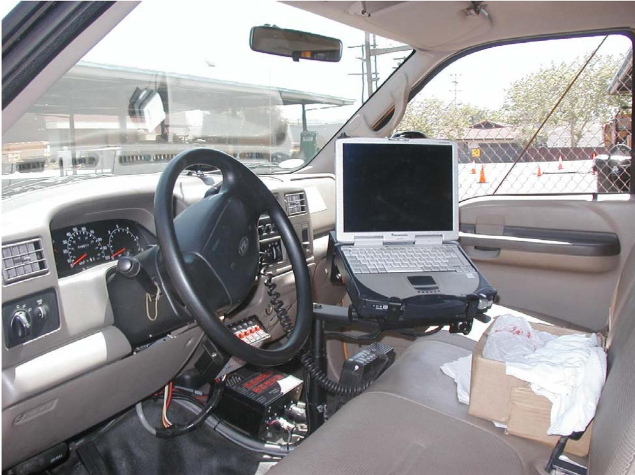
freely adjustable brackets that allow the computer to be used by either the driver or the passenger. Mounting hardware has been a special challenge because of the unusual configuration of the many special-purpose vehicles used, and the presence of controls for the complex hydraulic equipment.
